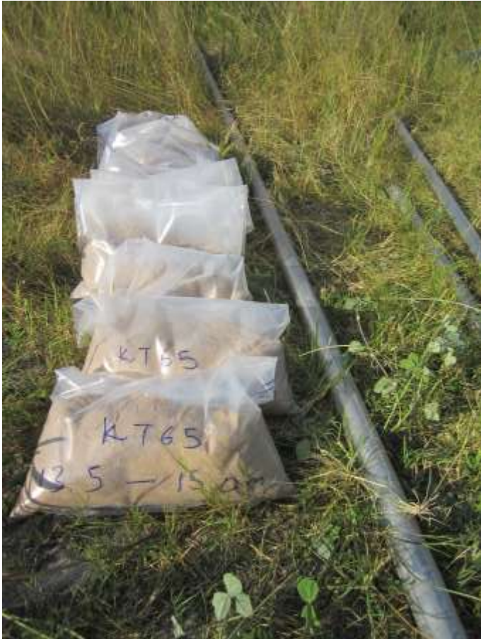
Figure 11-2 Sample collection with borehole ID and interval during power auger drilling
