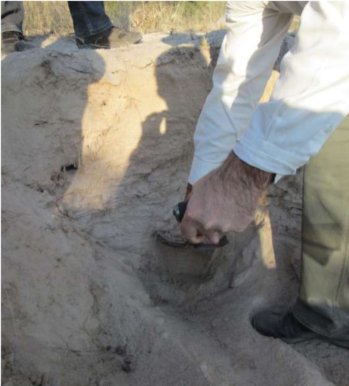
Figure 11-1 Sampling of pit wall using a shovel
