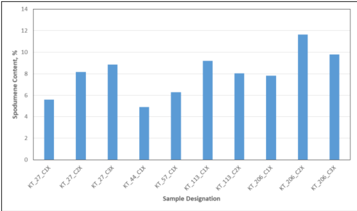
Figure 9-4 Abundance of spodumene in selected auger samples by assay validated Rietveld Refinement XRD (see also Table 9-2)
