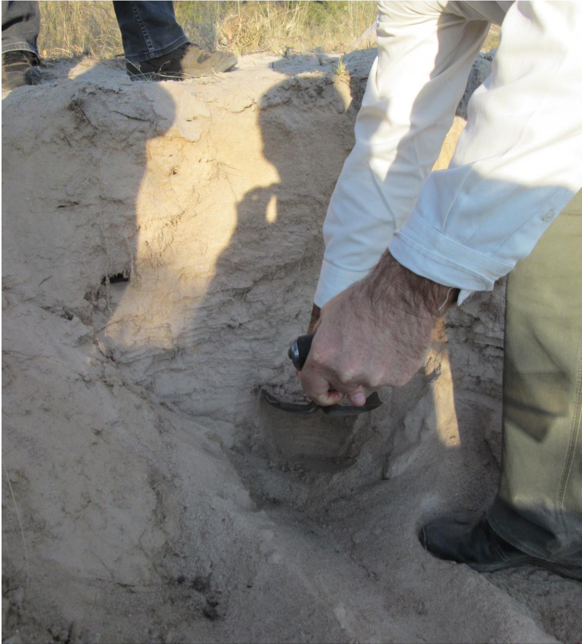
Figure 11-1 Sampling of pit wall using a shovel
