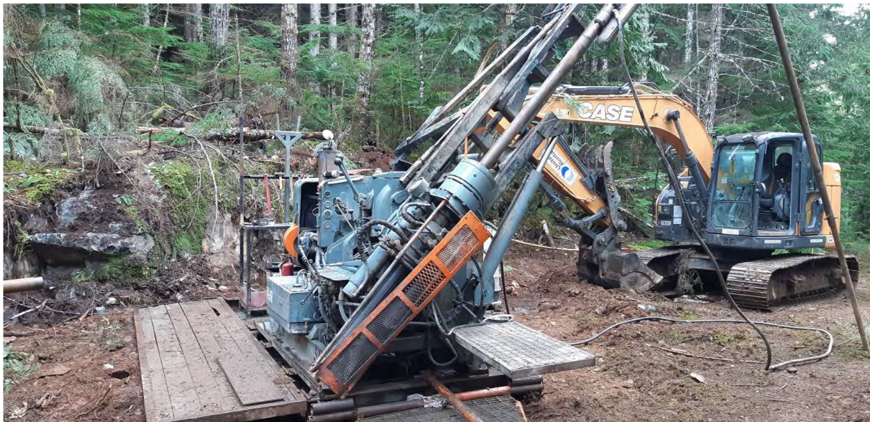
Figure 1 – Boyles 25 Diamond Drill on Setup #1 during previous drill campaign at Redonda Copper Project
