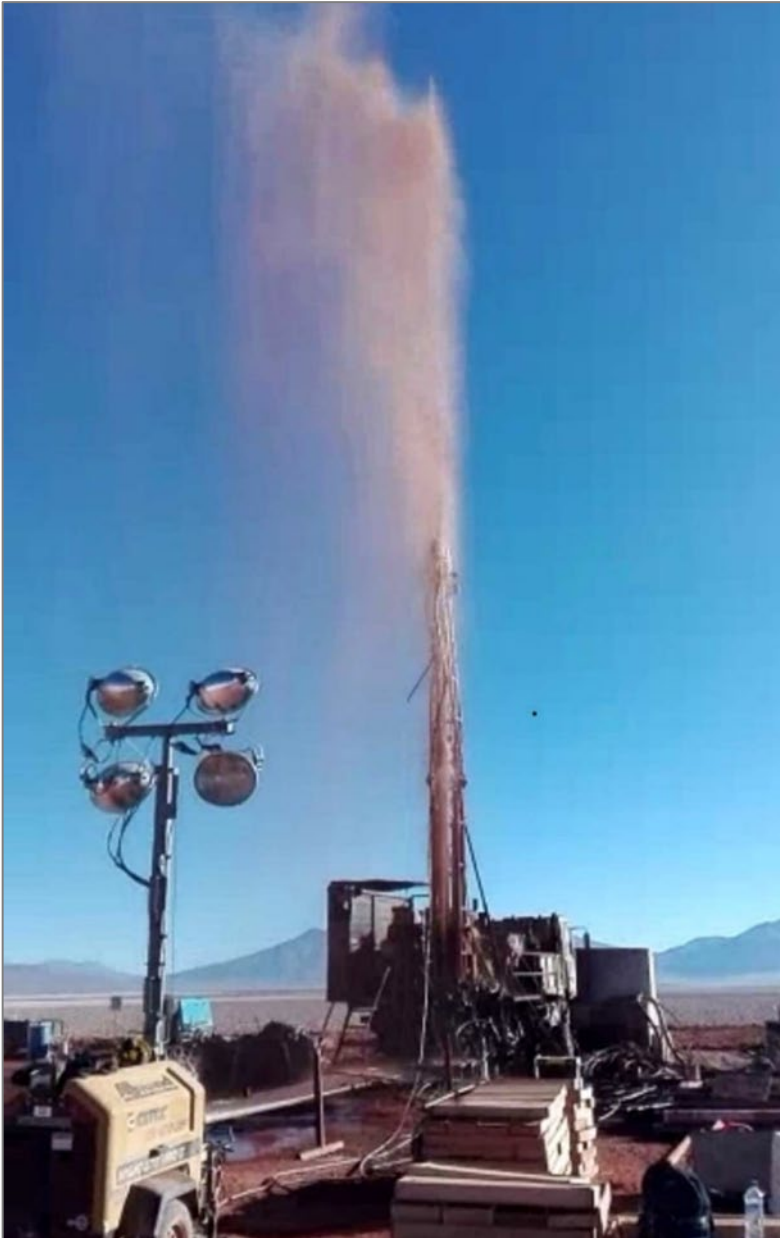
Figure 6.3 Brine surge from exploration well PCT-18-01 at approximately 355 m depth (Panopus, 2023)
