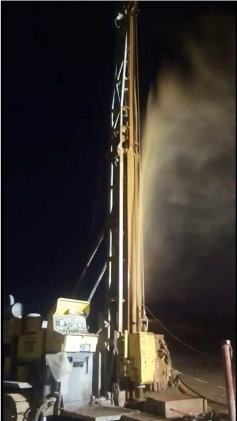
Figure 6.4 Brine surge from exploration well PCT-18-01 at approximately 355 m depth (Panopus, 2023)
