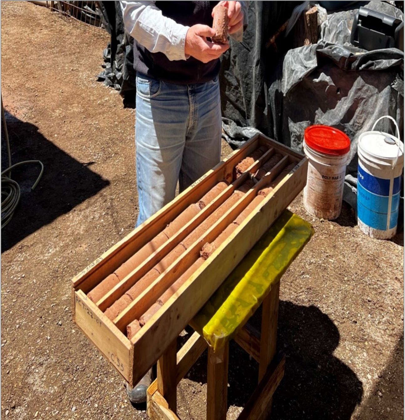
Figure 11.2 Phillip Thomas examining clay core recovered from exploration well PCT-22-01 at a depth of 200.05 m depth (Panopus, 2023)
