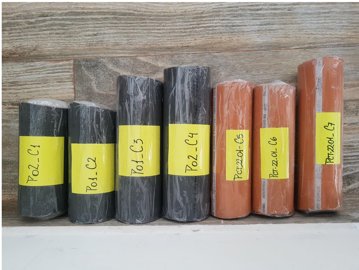
Figure 1 Sample cores ready for porosity and transmissivity tests
