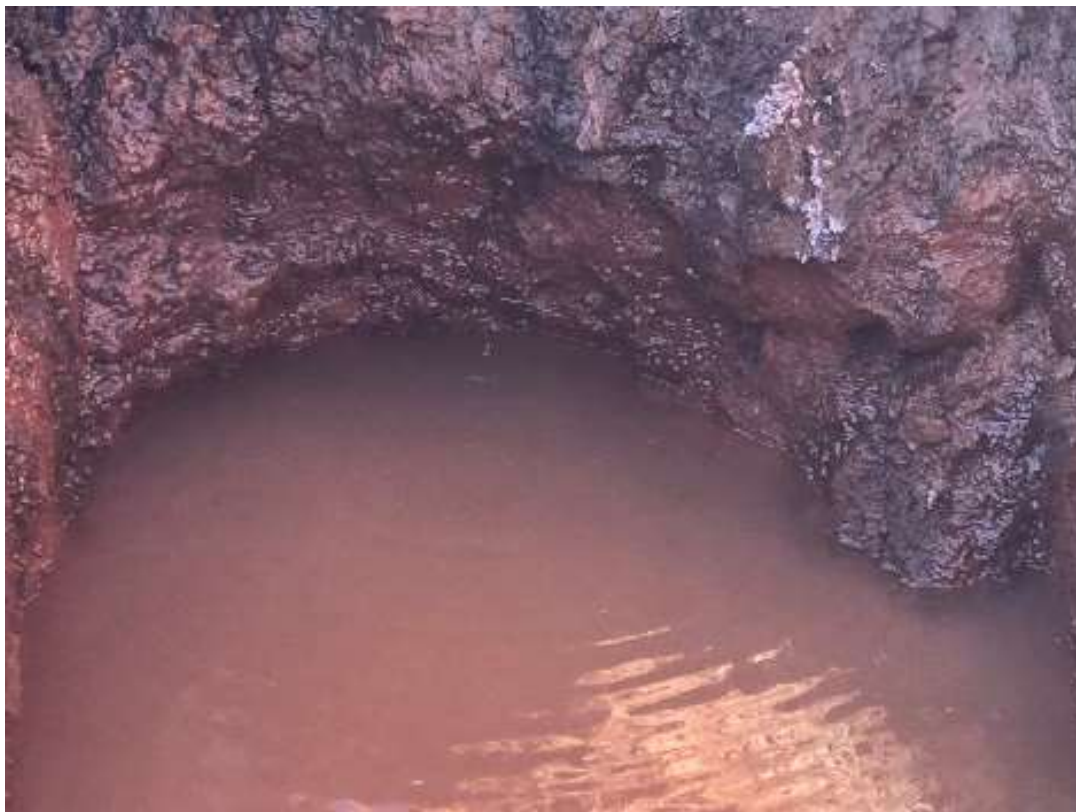
Figure 6-2 Picture of the trench Pit 1 with brine approximately 1 metre from the surface
