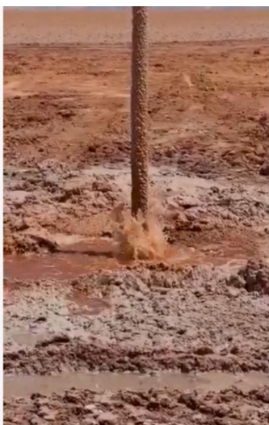
Fig 4. DDH1 brine flow with gas being released
