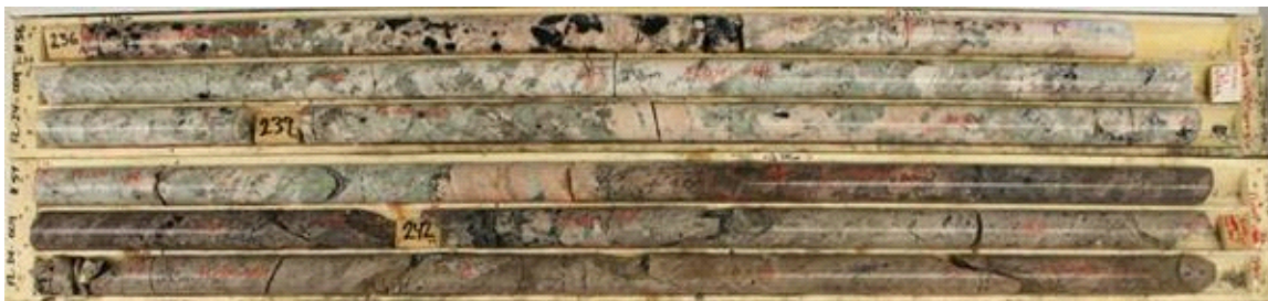
Pic 2. Spodumene Pegmatite from FL24-009. Approximately 1.52% Li 2 O over interval (235.98 m – 241.00 m)
