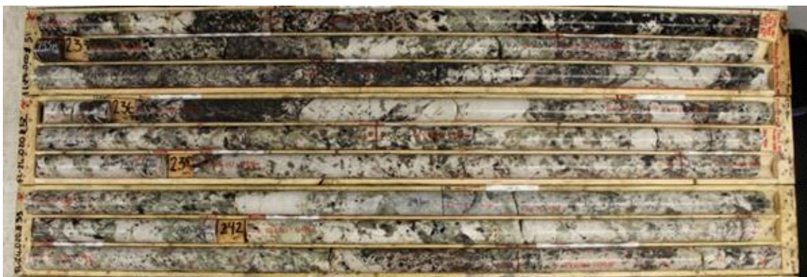
Pic 4. Spodumene Pegmatite from FL24-020. Approximately 0.75% Li 2 O over interval (232.00 m – 245.00 m)
