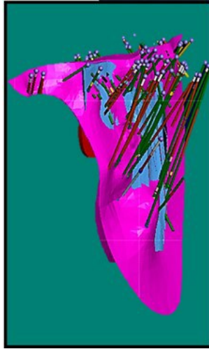
Figure 8 - 3-D Model of Dyke 1 with historic drillholes
