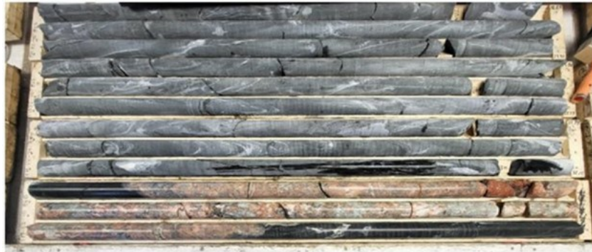
Figure 3. DDH FM22-70 drilled at -70 degrees inclination intersected two pegmatite dykes totaling 4.9 m with up to 15% light green spodumene crystal aggregates. The location of Dyke 16 is illustrated in relation to all previous pegmatite dykes on the Zoro property in Figure 4 below.
