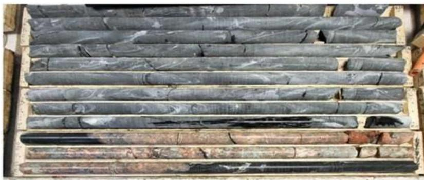
Figure 3. DDH FM22-70 drilled at -70 degrees inclination intersected two pegmatite dykes totaling 4.9 m with up to 15% light green spodumene crystal aggregates.
