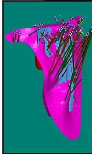
Figure 8 - 3-D Model of Dyke 1 with historic drillholes
