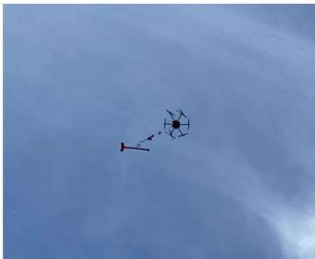
Picture 2. Drone Carrying a Magnetometer.
