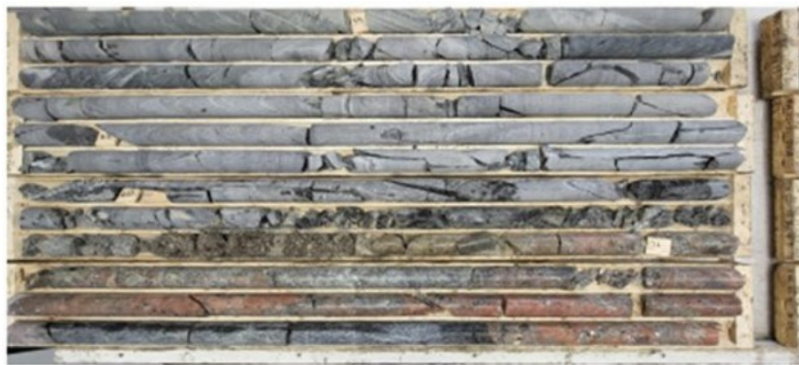
Figure 5. A 4.5 metre spodumene-bearing pegmatite was intersected between 70.45 and 75.89 m before being truncated by a fault.
