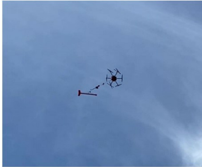
Picture 2. Drone Carrying a Magnetometer.
