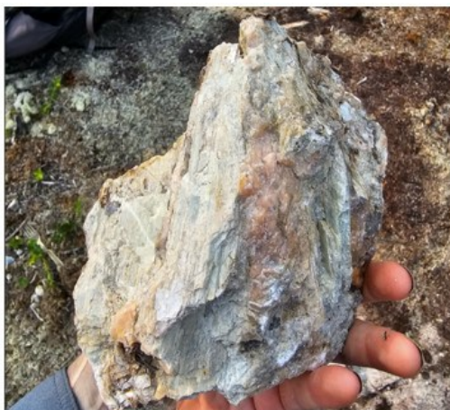
Picture 1. Large spodumene crystals found in outcrop at the B1 pegmatite; Sample 153026.
