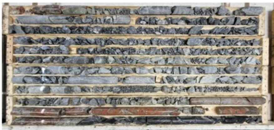
Figure 6. A further pegmatite was intersected below the fault between 84.4 and 86.65 m in Dyke 8.
