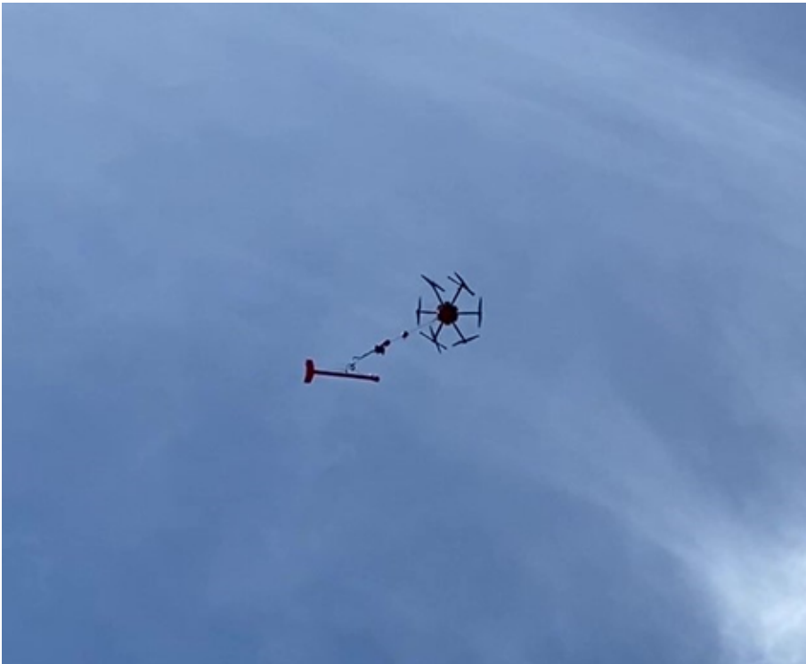
Figure 1. Drone Carrying a Magnetometer
