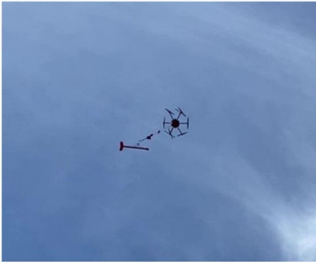
Figure 9. A magnetometer towed by a UAV or drone measuring the magnetic signature of the rocks on the ground over the Zoro Lithium Property.
