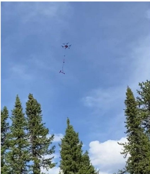
Figure 10. A magnetometer towed by a UAV or drone measuring the magnetic signature of the rocks on the ground over the Zoro Lithium Property.
