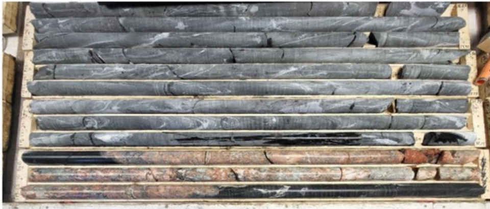
Figure 3. DDH FM22-70 drilled at -70 degrees inclination intersected two pegmatite dykes totalling 4.9 metres with up to 15% light green spodumene crystal aggregates. The location of dyke 16 is illustrated in relation to all previous pegmatite dykes on the Zoro property in Figure 4 below.
