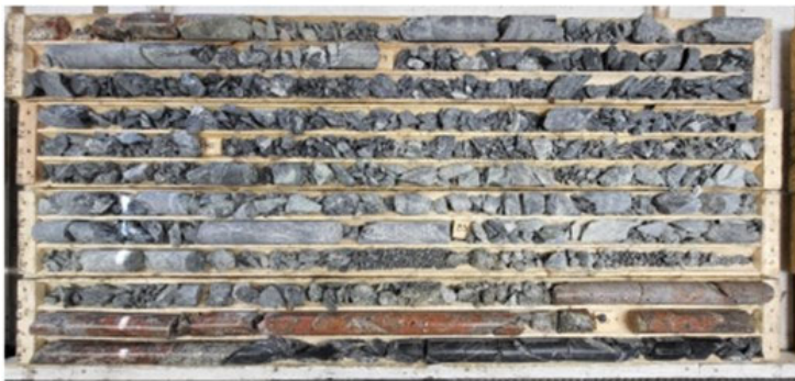
Figure 6. A further pegmatite was intersected below the fault between 84.4 and 86.65 metres in Dyke 8.
