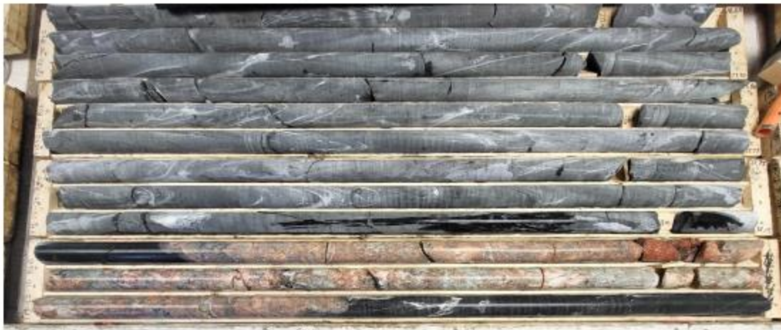
Figure 3. DDH FM22-70 drilled at -70 degrees inclination intersected two pegmatite dykes totalling 4.9 metres with up to 15% light green spodumene crystal aggregates.
