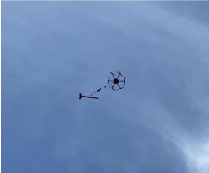
Figure 10. A magnetometer towed by a UAV or drone measuring the magnetic signature of the rocks on the ground over the Zoro Lithium Property.
