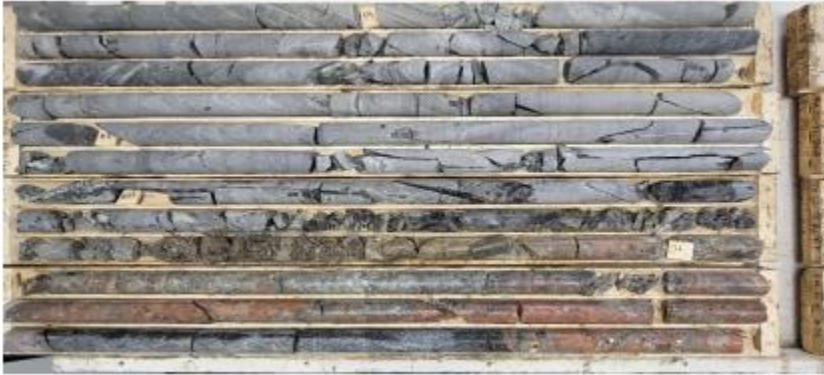
Figure 5. A 4.5 metre spodumene-bearing pegmatite was intersected between 70.45 and 75.89 metres before being truncated by a fault.
