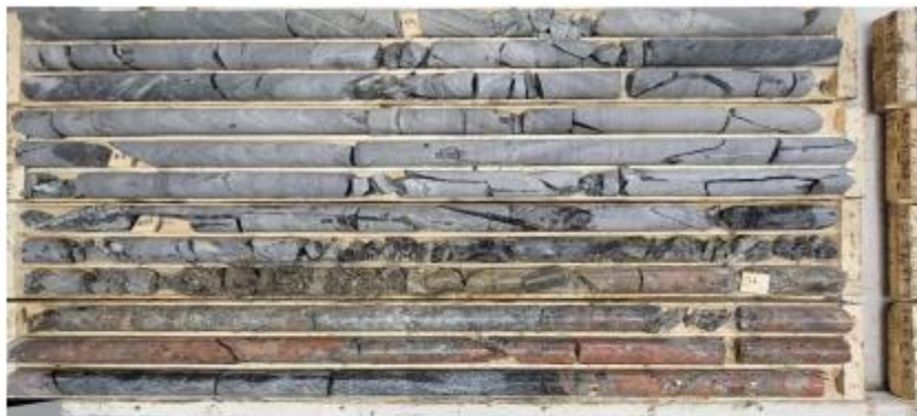
Figure 3 - A 4.5-meter spodumene-bearing pegmatite was intersected between 70.45 and 75.89 meters before being truncated by a fault
