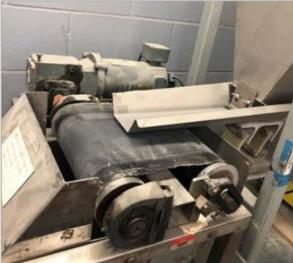
Figure 1: High-Force® Dry Magnetic Separator Used for HLS Sinks and DMS Concentrate
