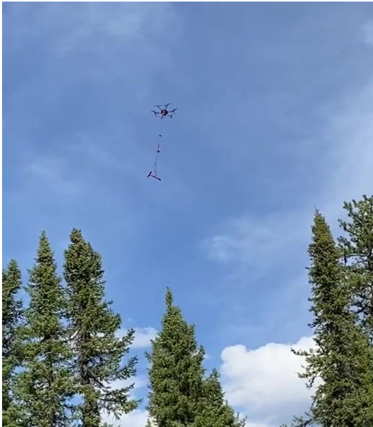
Figures one and two show a magnetometer measuring the magnetic signature of the rocks on the ground over the Zoro Lithium Property.
