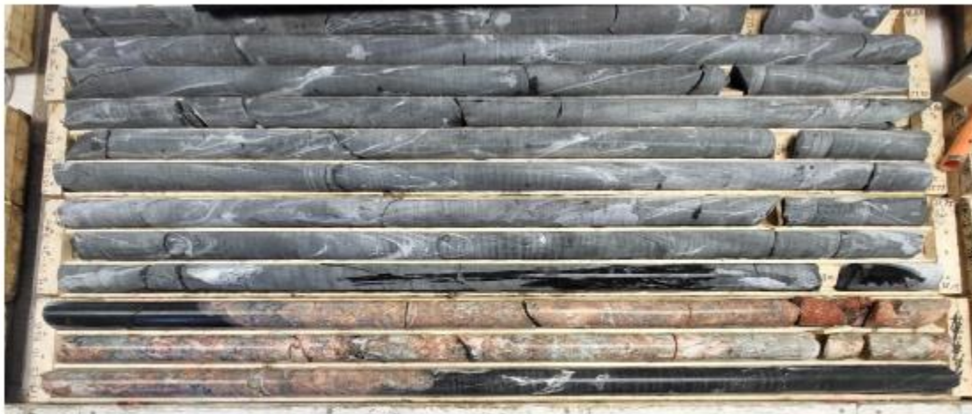
Figure 1 - DDH FM22-70 drilled at -50 degrees inclination intersected two pegmatite intercepts totaling 4.9 meters with up to 15% light green spodumene crystal aggregates.
