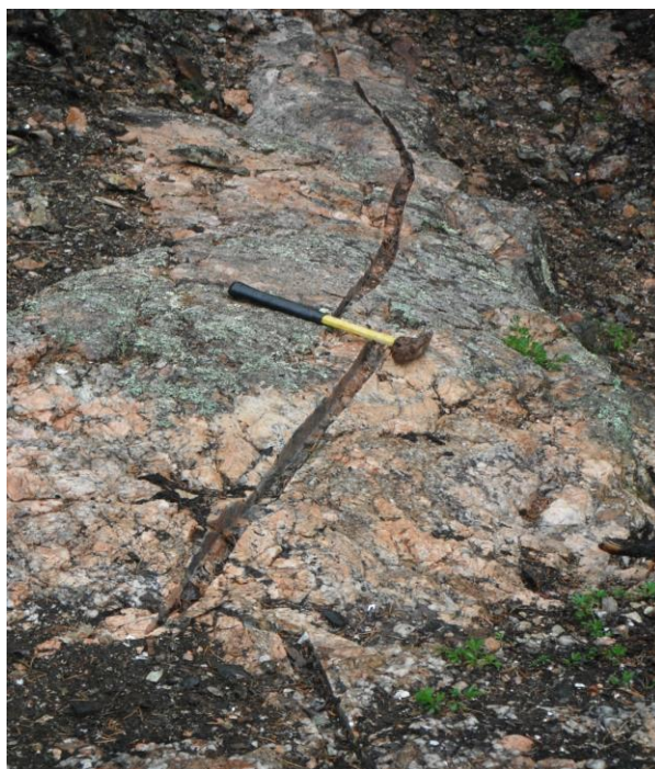
Figure 11.3.1: Channel cut for sampling of the Zoro 1 spodumene pegmatite.
