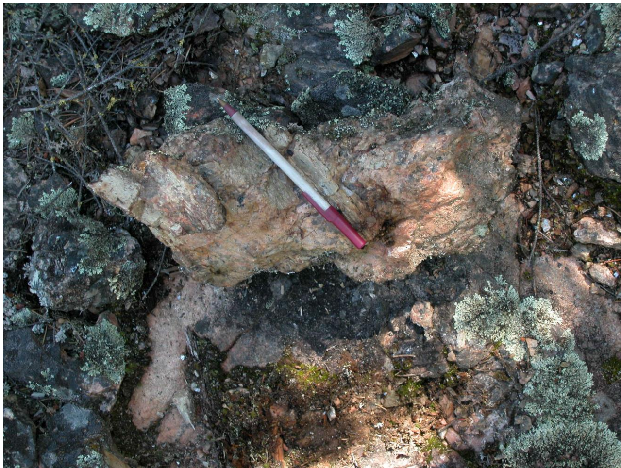
Figure 7.6.1: Coarse-grained bladed spodumene, trench muck sample, Dyke 1, Zoro Lithium Project.
