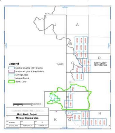
The claim block corners and boundaries are marked with posts, blazing and flagging according to the regulations of the Northwest and Yukon Territories. Post and line locations were established by handheld GPS readings. Several lines were observed by the Author and they appear to be properly established.
