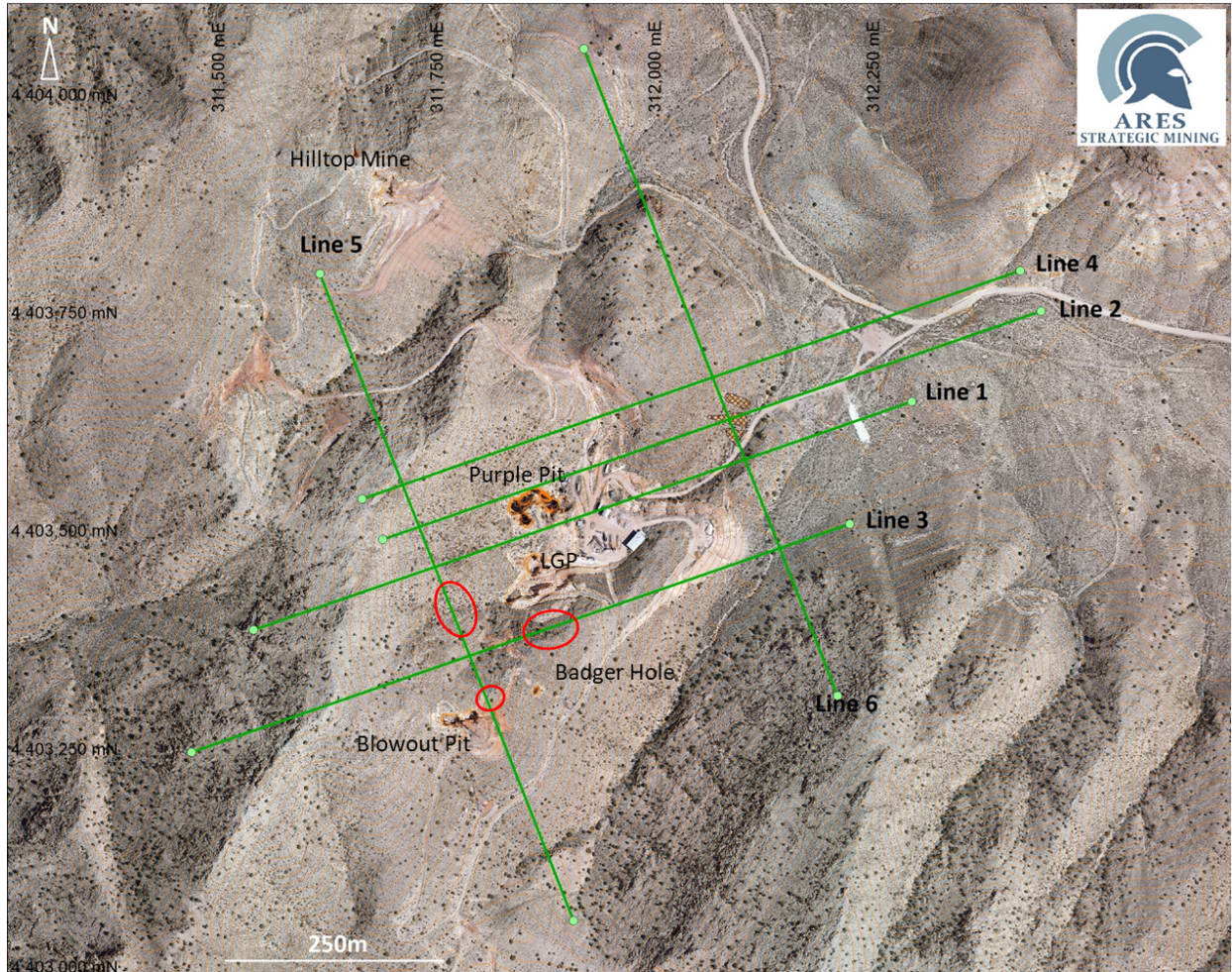
Figure 1. Location of IP section lines, and position of the newly located breccia pipes (red circled areas)
