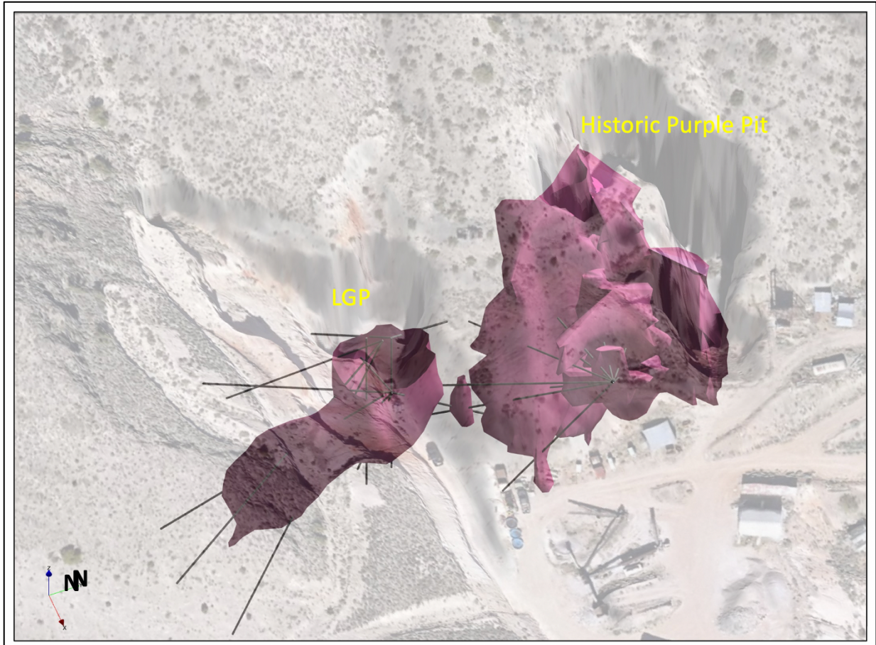
Figure 6. Preliminary 3D render of the Fluorspar mineralization distribution after completion of 2020 delineation drilling at the Lost Sheep Mine (see buildings for scale).
