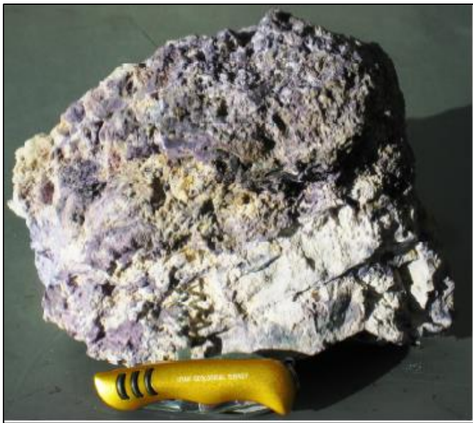
Fig. 13. Fluorite-chalcedony-bertrandite Be ore nodule from an open pit at Materion's (Brush Wellman) Spor Mountain operation, Juab County (3 inch pocket knife for scale).
