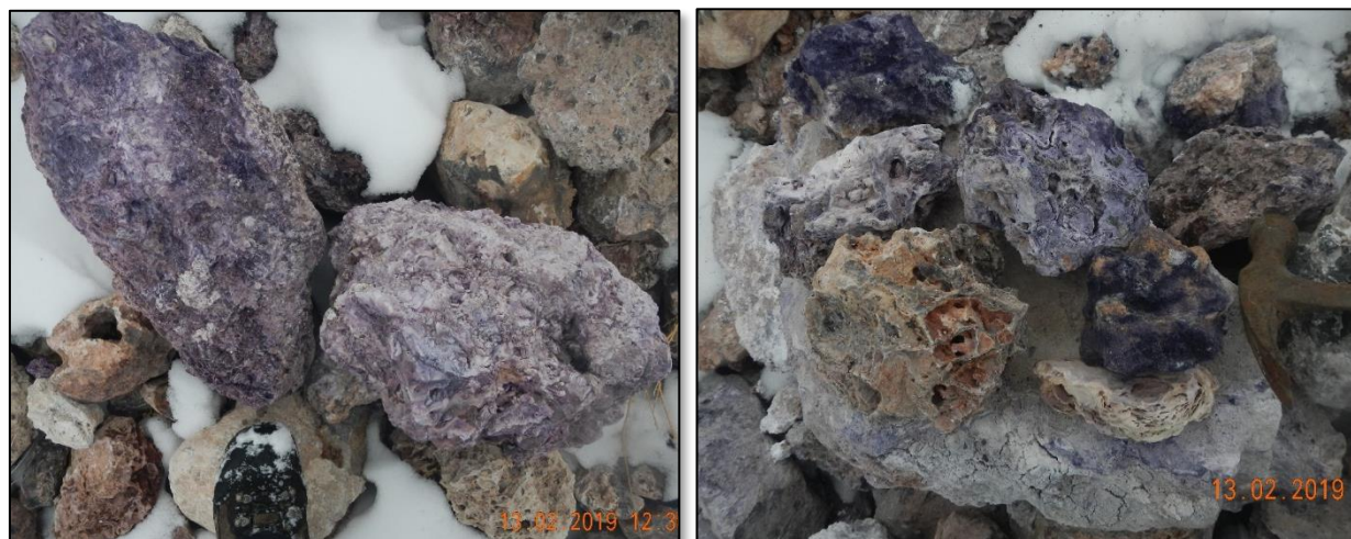
Figs. 16 & 17. Fluorspar mineralisation, LSM with foot and claw hammer for scale. Weathered material is paler with freshly broken ore mauve to deep purple. Note strong fluorite-clay-silica-(calcite) open space mineralisation and wavy, undulose, boxwork and vuggy textures from carbonate dissolution and replacement.
