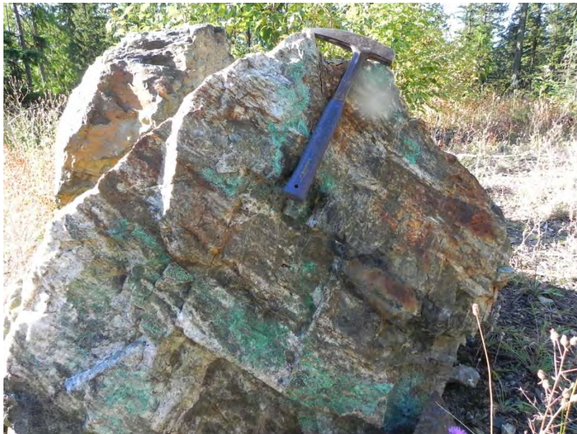
Photo 1: North Showing (Zappa Trench). Boulder of quartz-rich amphibolite with chalcopyrite and pyrite-bearing horizons. Possible stratabound exhalative mineralization.
