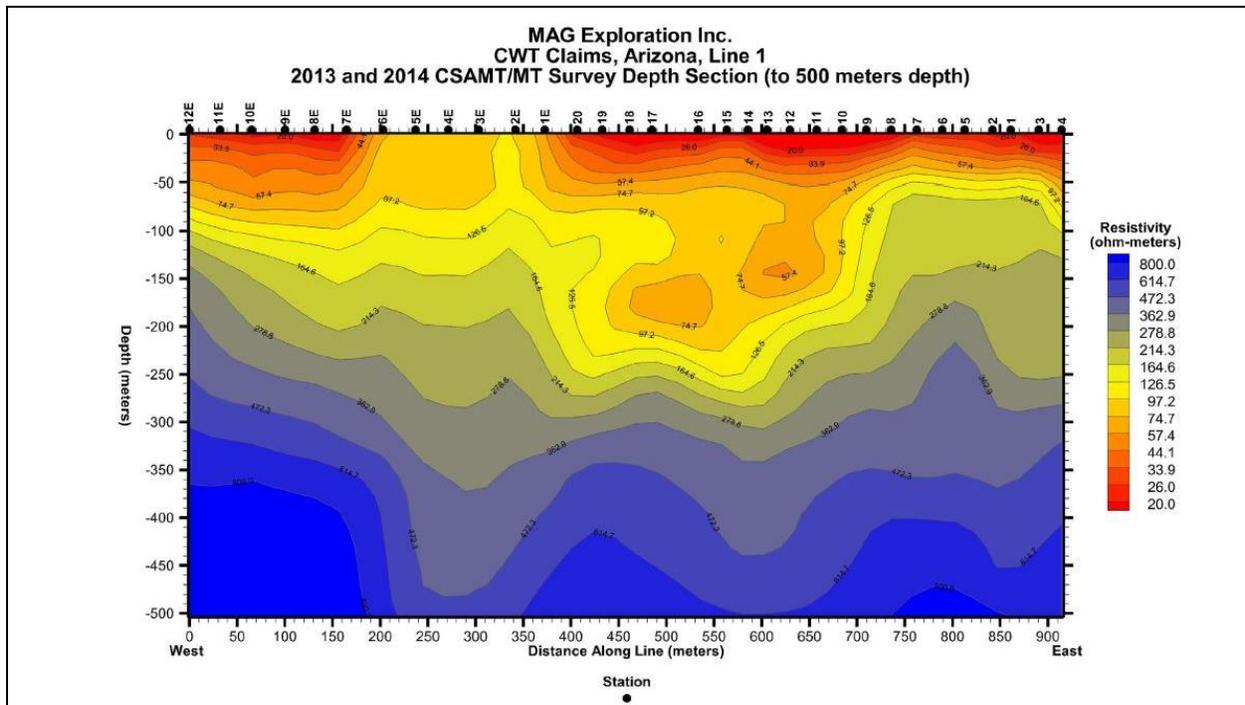
Figure 10a. CSAMT-MT Line 1 Depth Section
