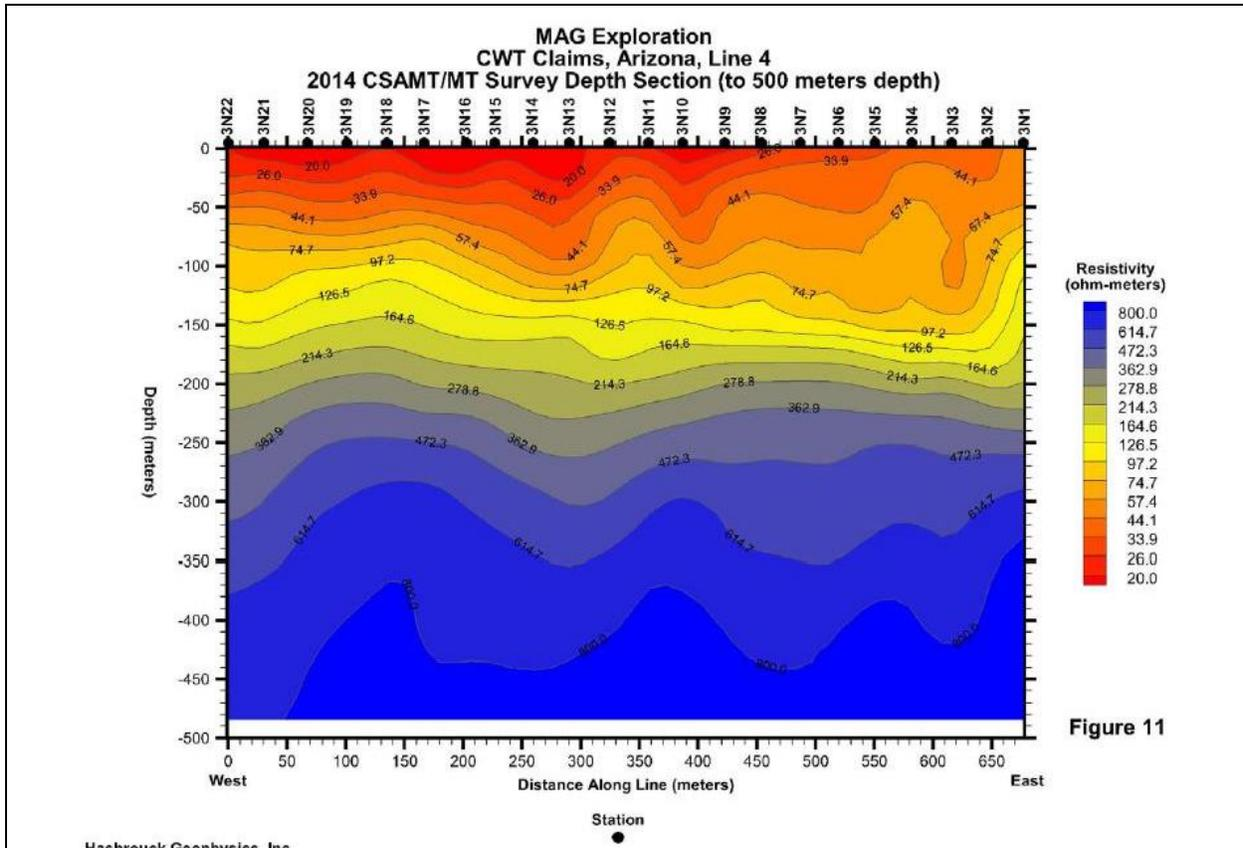
Figure 10d. CSAMT-MT Line 4 Depth Section
