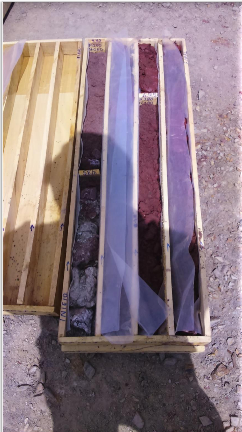
PICTURE 10.3 TAILINGS MATERIAL IN CORE BOXES
