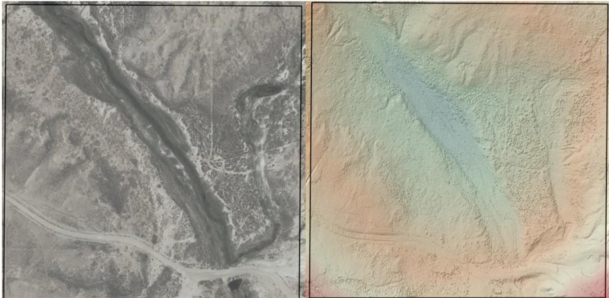
Figure 2 Example of high-resolution Data Elevation Model on Big Bend claim. Left: Publicly available satellite imagery (Bing, 2024); Right: Hill-shaded and coloured DEM image from 2024 drone survey.
