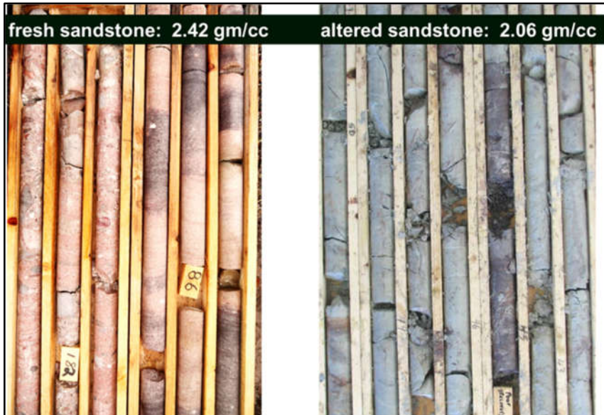
Figure 9: Fresh and Clay Altered or Argillized Sandstone
