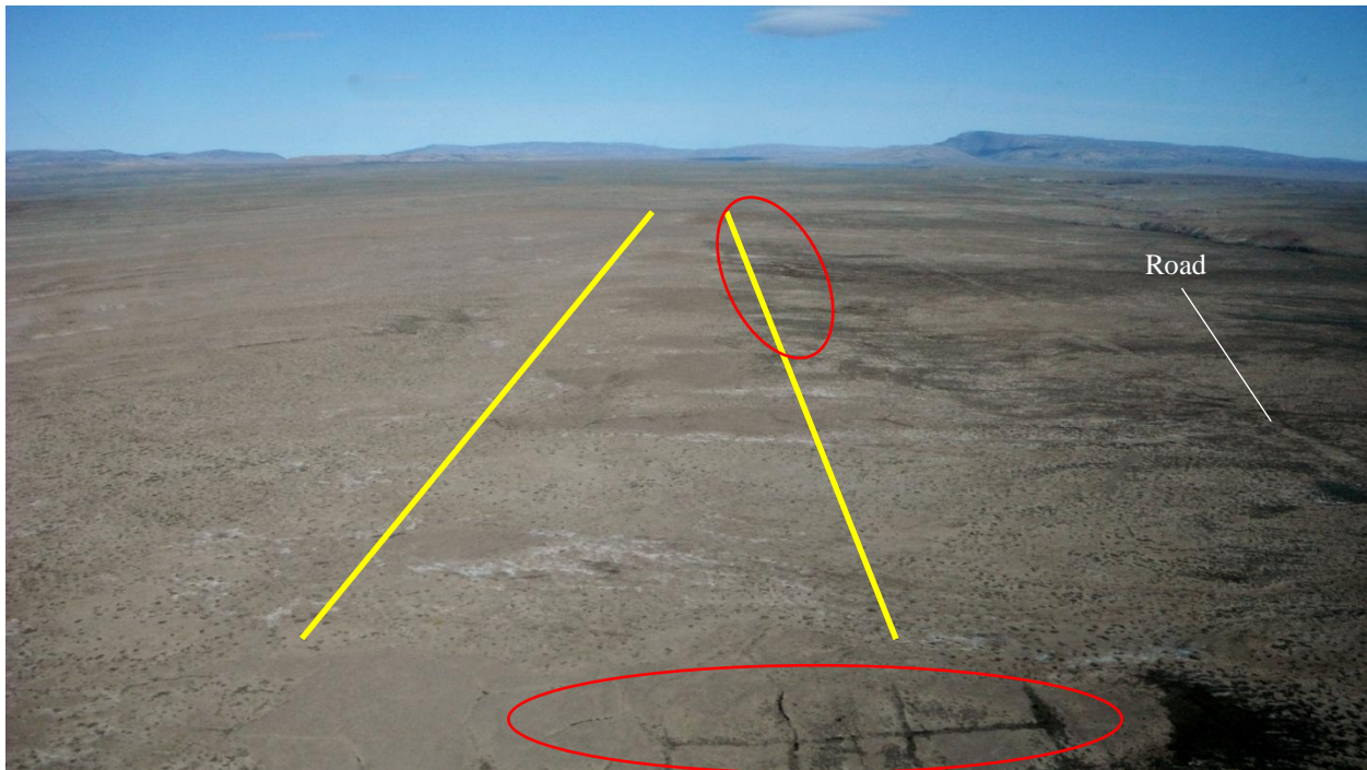
Figure 12.6: Aerial view looking northwest from the southern end of the runway. The approximate extent of data coverage and estimated edge of runway is identified in yellow. The approximate location of ice wedge polygons is identified in red. Note the patchy appearance of the darker drifted sandy material, and also a road to the east (right in picture) running parallel to the proposed runway.
