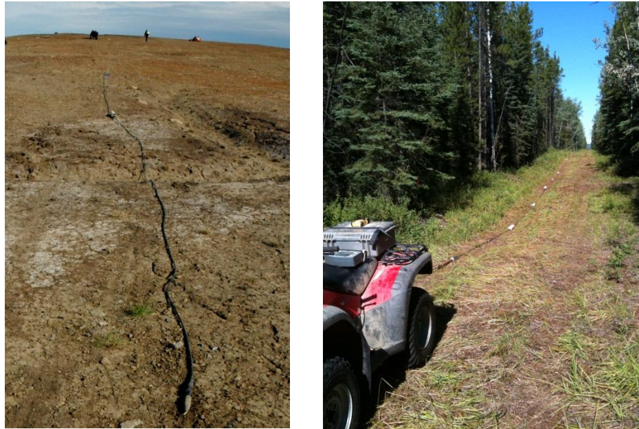
Figure 12.18: OhmMapper system setup. 10 metre cable arrangement from behind at the Ellesmere location (Left).
