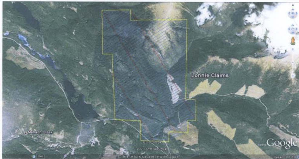
Figure 2: Airborne geophysical survey lines in blue, tie lines in red and the boundary in yellow.
