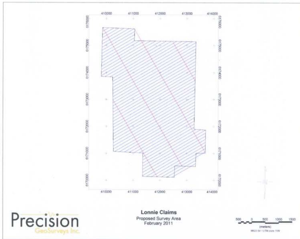
Figure 3: Proposed survey basemap with survey lines in blue and tie lines outlined in red and the boundary in black. The Easternmost proposed tie line was not completed due to poor weather conditions.
