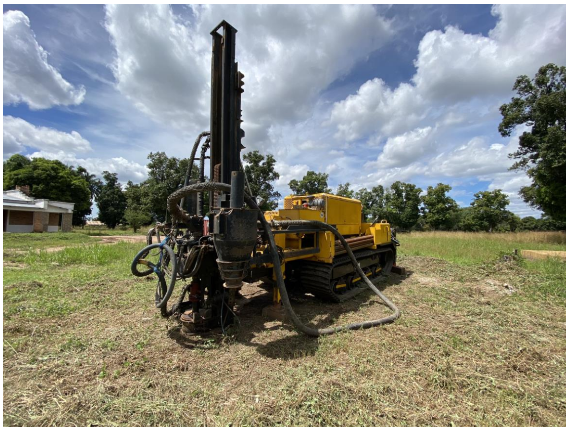
Figure 11-3 Track mounted aircore rig with mounted cyclone
