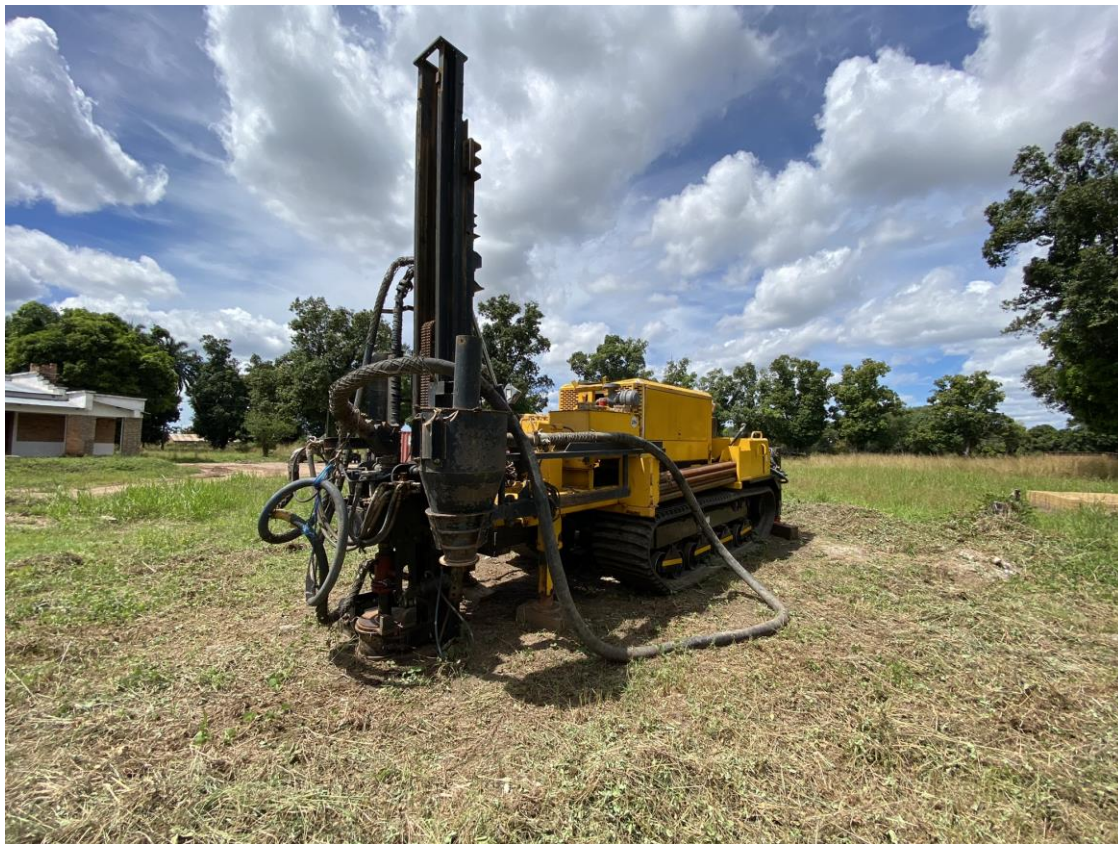
Figure 11-3 Track mounted aircore rig with mounted cyclone
