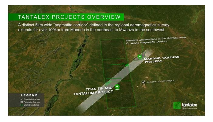
The TiTan plant is located just south of the Pegmatite Corridor in an ancient riverbed. Coltan and cassiterite is found in gravel layers 1-2 meters thick under approximately 7m of overburden.
