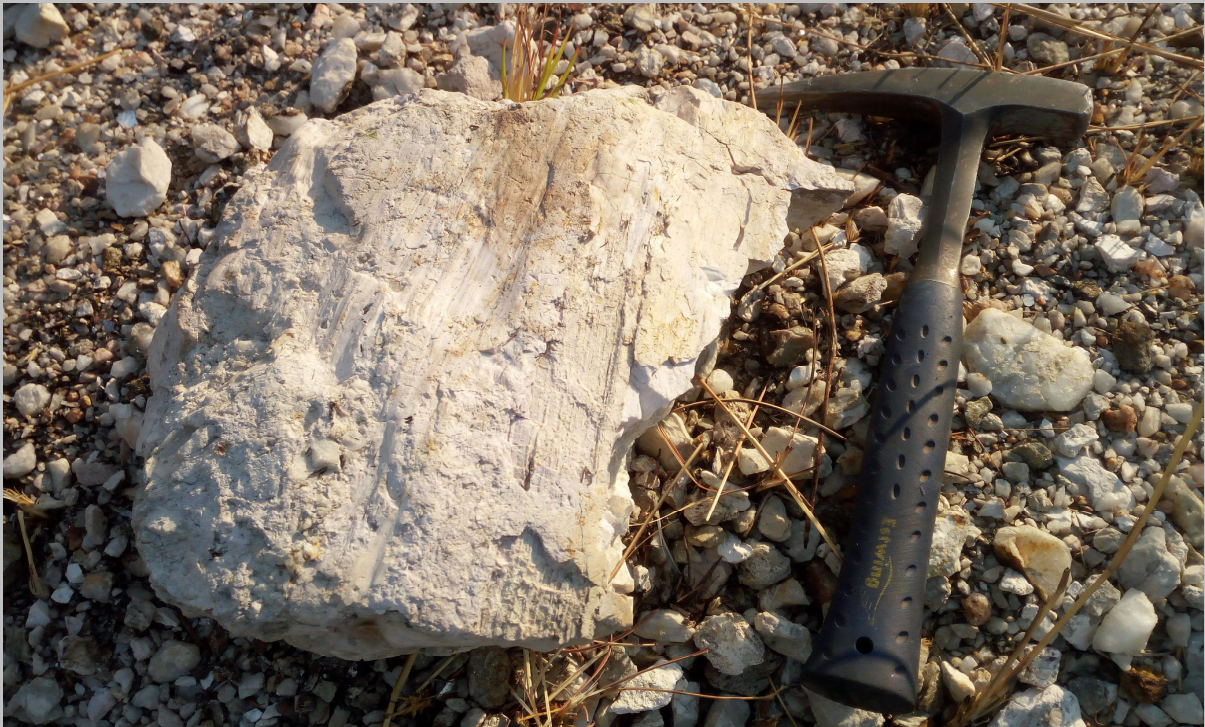
Figure 7.3 Pegmatite from the Manono – Kitolo pegmatites showing distinct spodumene pseudomorphs set in a quartz – albite rich matrix.
