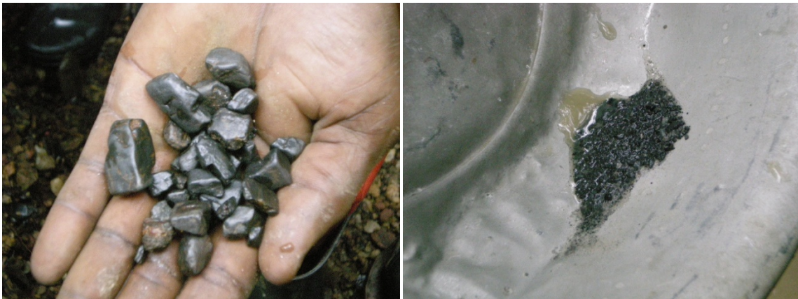
Picture 11: Coltan pebbles collected at site 88040008 and pan concentrates collected at site 88040001. Note that the pebbles were subsequently assayed in laboratory with a portable XRF analyser by the author and confirmed as coltan.
