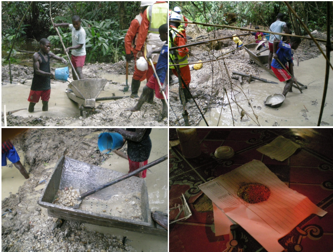
Picture 7: Views of the artisanal gold mining operations using sluice boxes operated by children. The method is identical to the one used by Avoine Mining, but without bypass channels and dam. The last picture shows gold concentrate being traded at the village maki.
