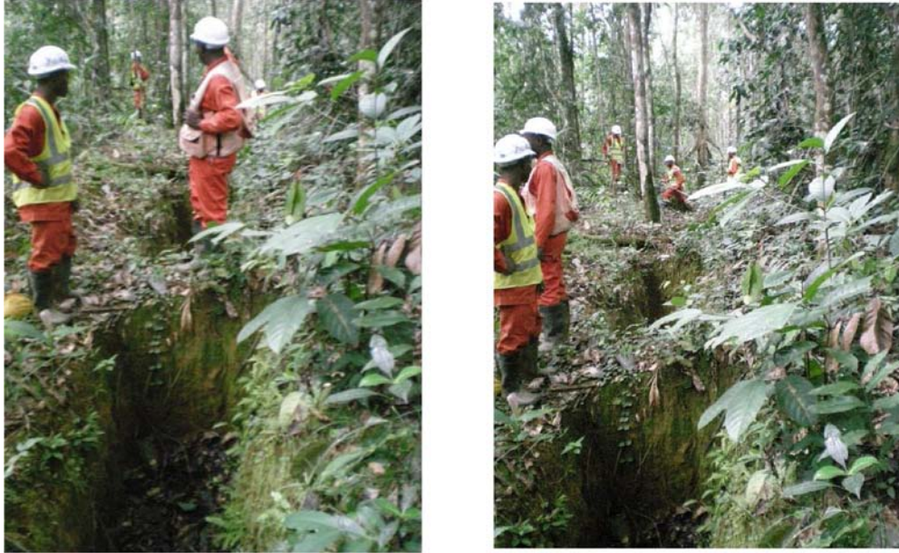
Picture 17: A series of small exploration pits dug for gold by Sino-Congo near a former Société Avoine exploitation (site 88040021).
