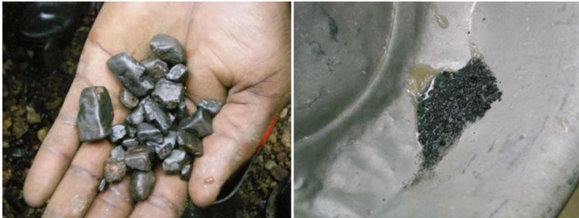
Picture 11: Coltan pebbles collected at site 88040008 and pan concentrates collected at site 88040001. Note that the pebbles were subsequently assayed in laboratory with a portable XRF analyzer by the author and confirmed as coltan.
