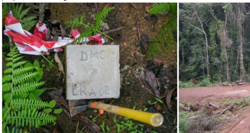
Picture 16: Concrete slab sealing off DMC’s (African Iron Ore) reverse circulation drill hole, and Congo Mining’s (Equatorial Resources) drill site with samples. Both operations are located close to a stream containing coltan.
