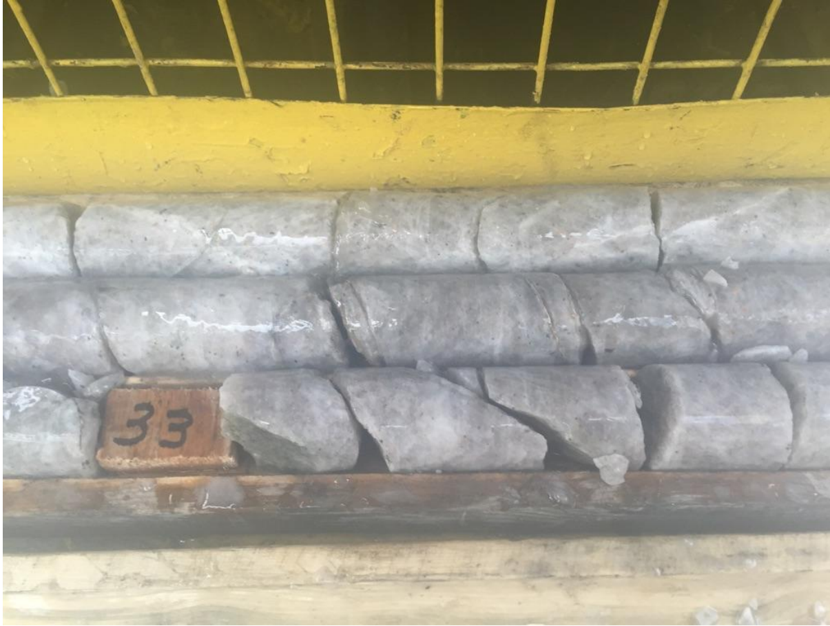
Photo 2 Typical Quartzite in Drillcore at Zone D
