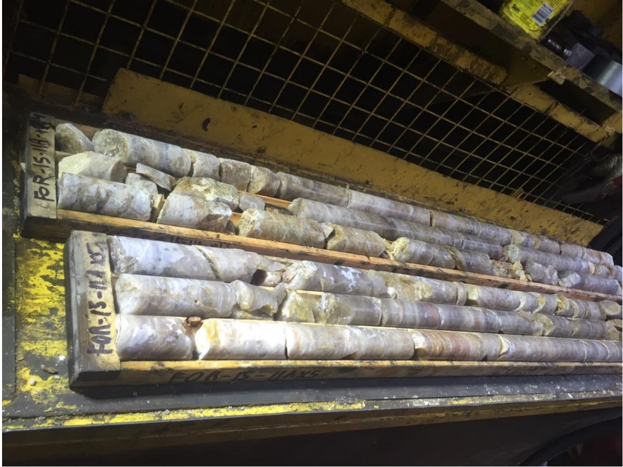
Photo 5 Typical Quartzite from Zone A Drilling
