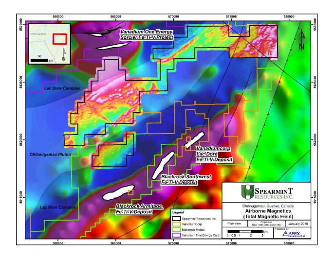
During November and December, 2018, the Company commissioned Calgary, Alberta based Earth Scan Technologies Ltd. to complete drone and heli-borne airborne magnetic geophysical surveys totaling 932 line-km over an area totalling approximately 3,400 hectares at 100 metre line-spacing.
