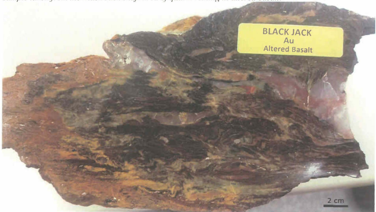
Figure 4.20 - Picture of sample at the Ontario Geologic Survey's Kenora office of a cut and polished sample taken from the Black Jack shaft area of quartz veining in altered basalt.
