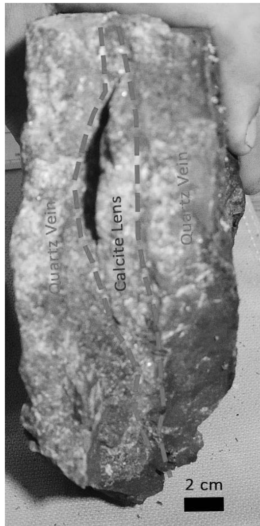
Figure 7.7 Sample ID K934654 from Black Jack North showing a carbonate lens with vuggy contact bound by quartz vein material.
