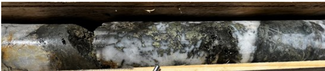
Figure 2 & 3: Chalcopyrite primary mineralization FAR-22-020 from 6m wide zone at 145.5m and 147.5m
