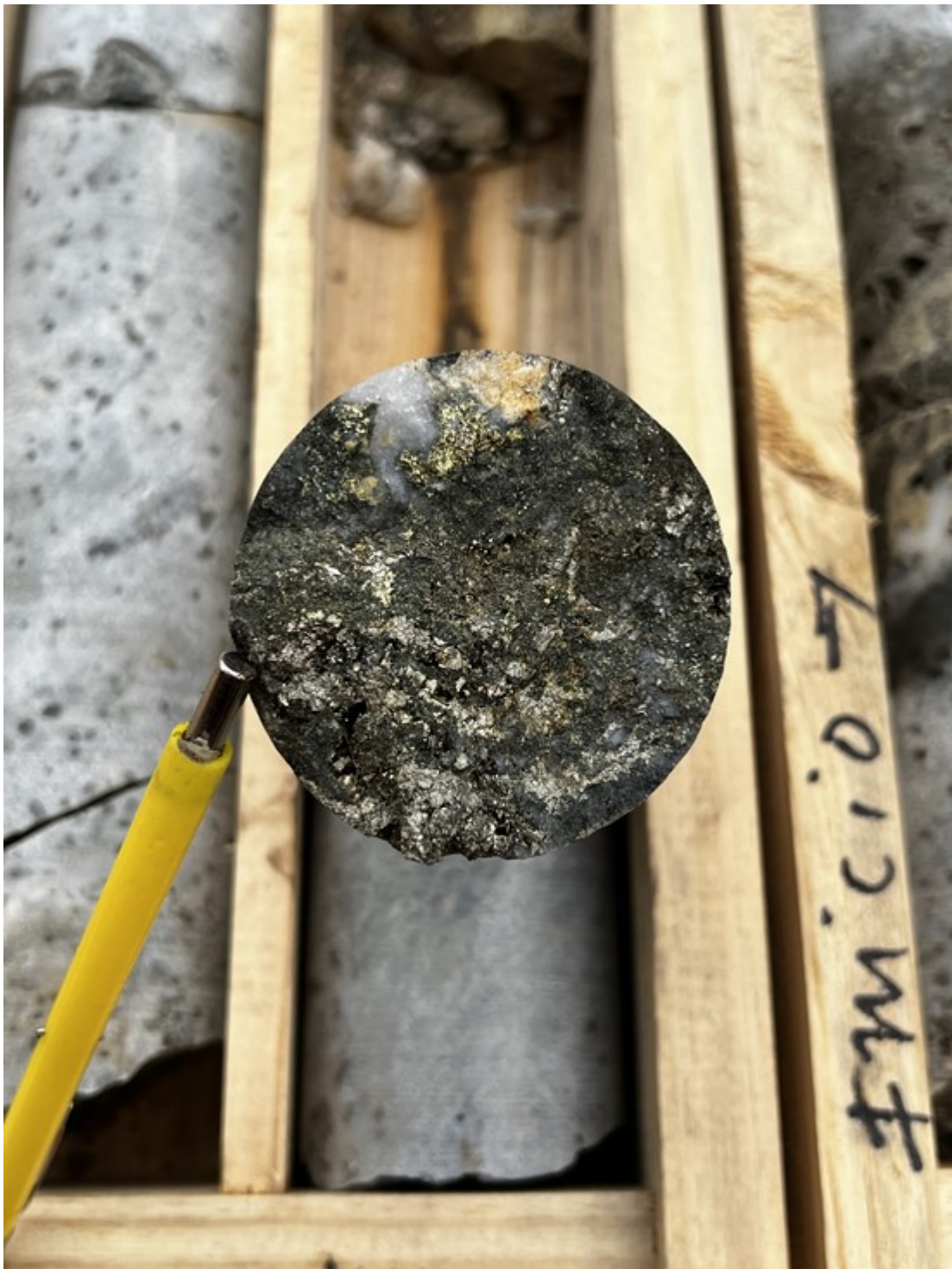
Figure 1: Chalcopryite, pyrrhotite and pyrite in quartz vein FAR-22-012
