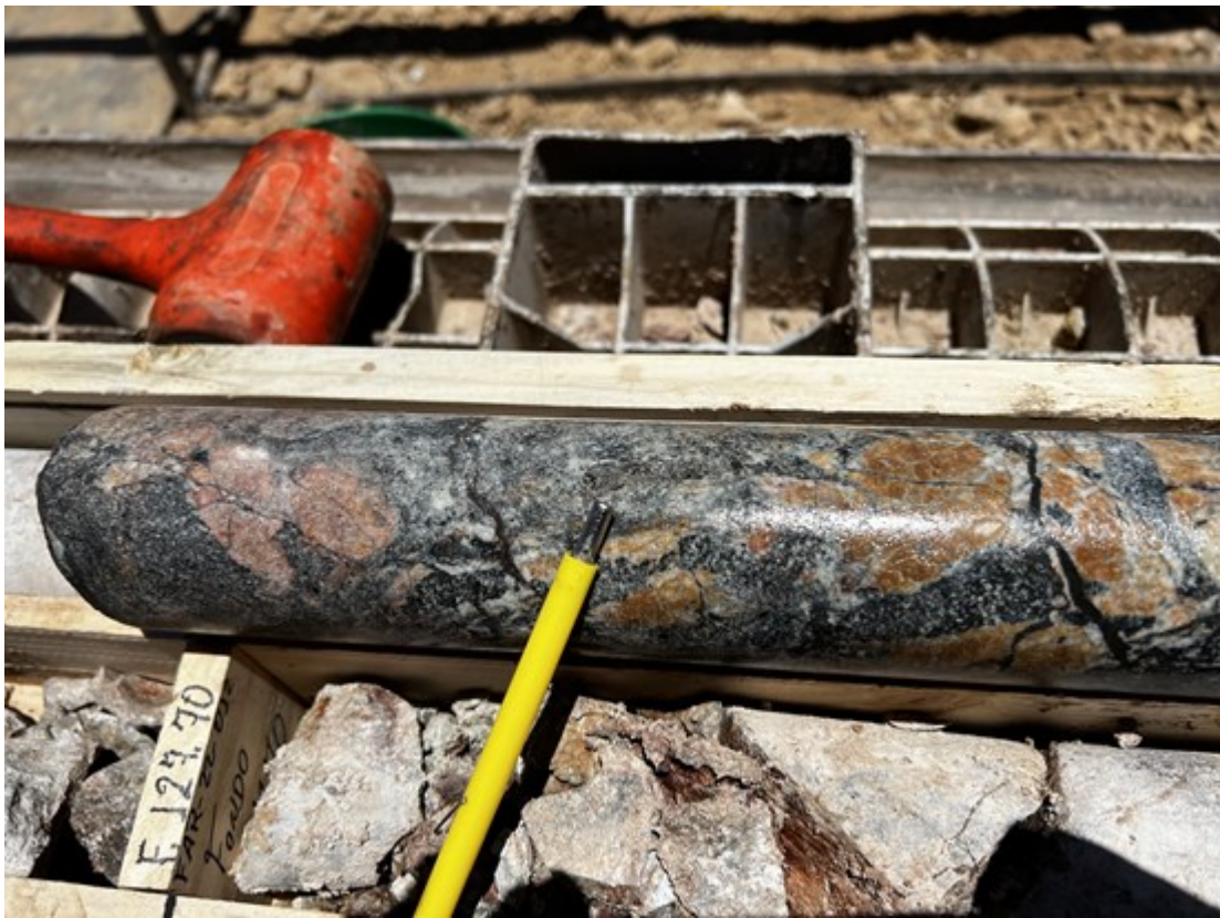
Figure 2: Brecciated structures with potassic alteration FAR-22-12
