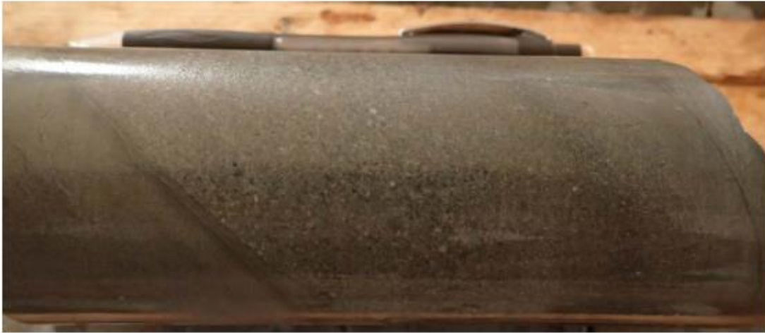
Figure 7-5: Bedded Sandstone in drillhole ORPD108 at 173 m
