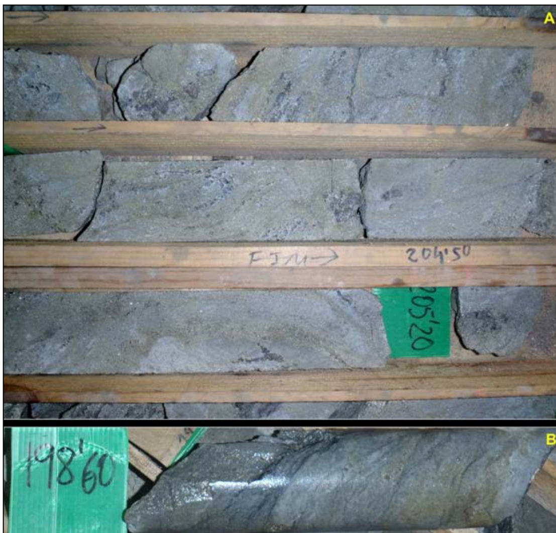
Figure 6-18: Photos to show the similarity of planar features in sulphide-bearing zones with those developed in unmineralised shear zones. Photo “A” shows diamond hole ORPD_11 at approximately 204 m. A shear zone showing similar ductile deformation features but an absence of sulphide mineralisation is shown in photo “B”, intersection taken from diamond hole ORPD_11 at 198.6 m. (Source: Olinda)
