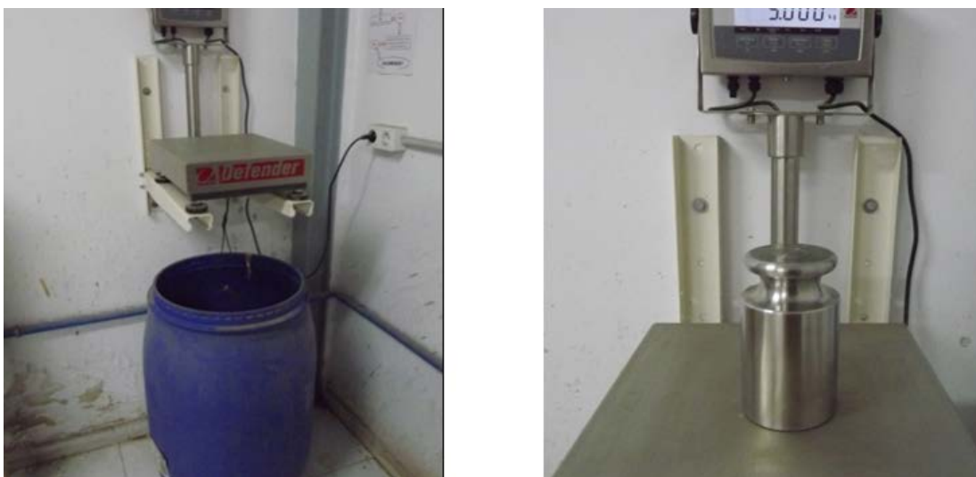
Figure 10-2: MESPA density determination equipment showing the scale and water immersion tub (left) and the calibration process (right)
