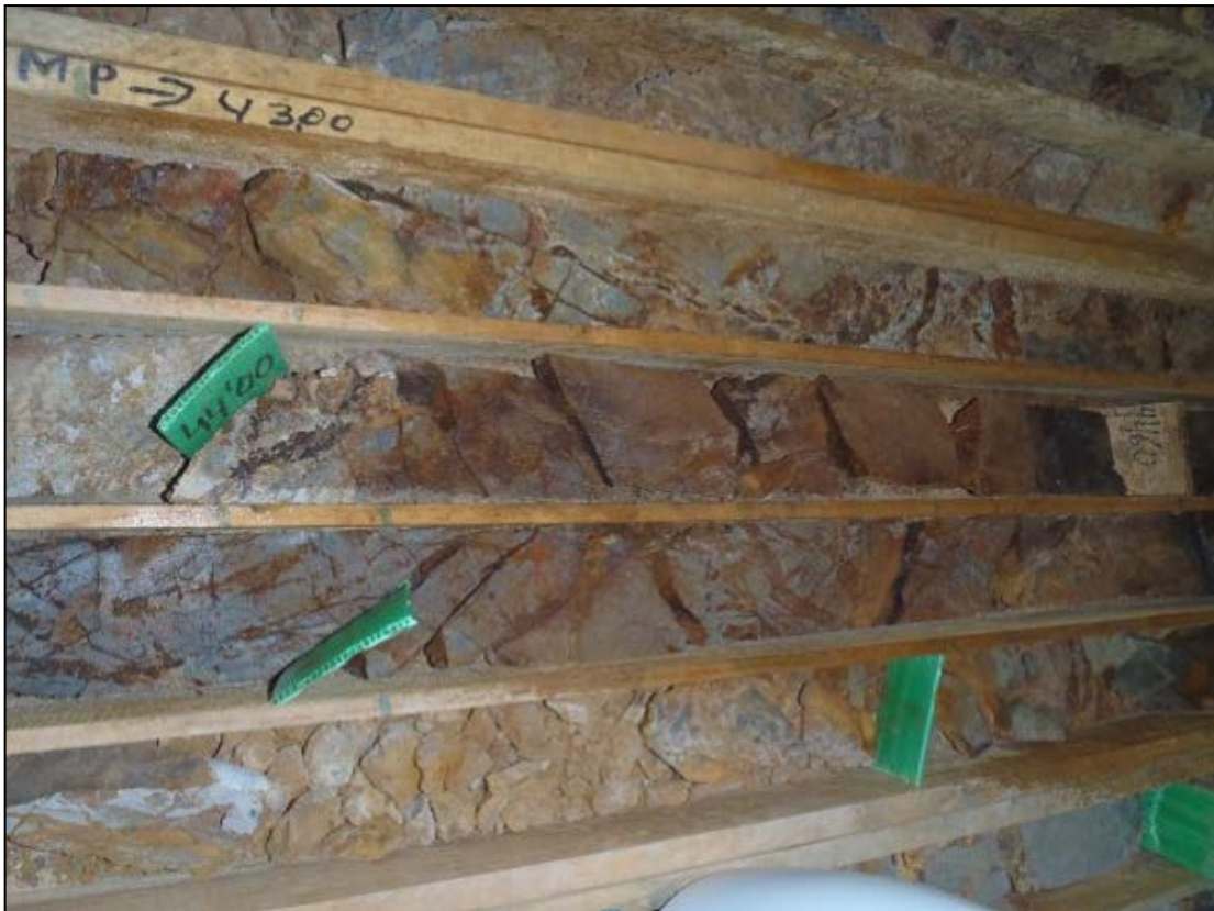
Figure 6-17: Sn mineralized structure showing strong iron-coated fractures. Diamond hole ORPC_02 at 44 m (Source: Olinda)
