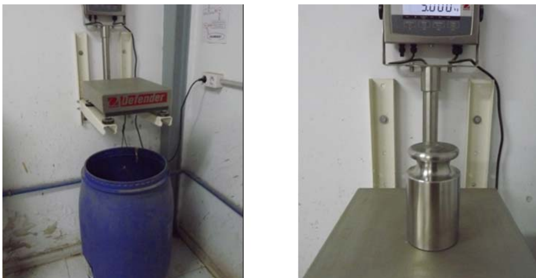
Figure 10-2: MESPA density determination equipment showing the scale and water immersion tub (left) and the calibration process (right)
