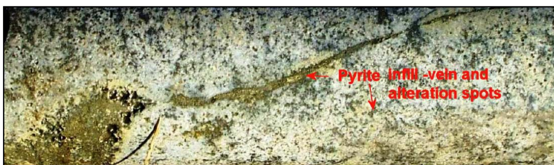
Figure 6-34: Pyrite vein with associated spot alteration of “sandstone”. (ORPCB, 191.3 m) (Source: Roger Taylor)
