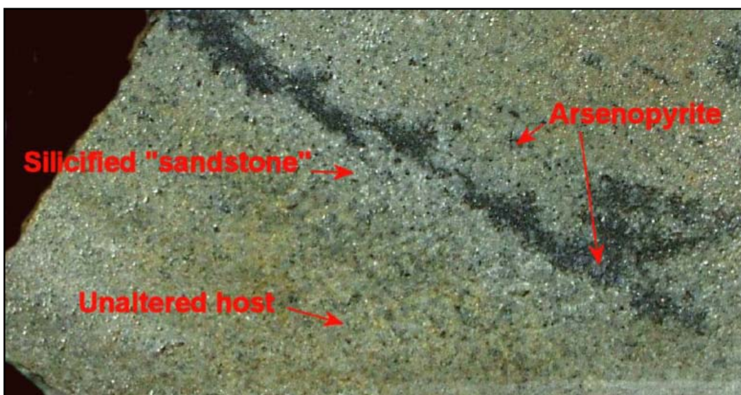
Figure 6-24: Arsenopyrite veinlet with subtle silicification halo. Note dark silica immediately adjacent to arsenopyrite (ORPC4, 122.45 m) (Source: Roger Taylor)
