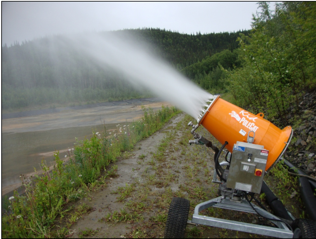
Figure 6: Evaporation Mister at Tailings Pond
