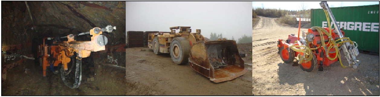
Figure 3: Mine Equipment Purchases (L to R: One Boom Jumbo, 4 yd 3 Scooptram, LH Drill)
