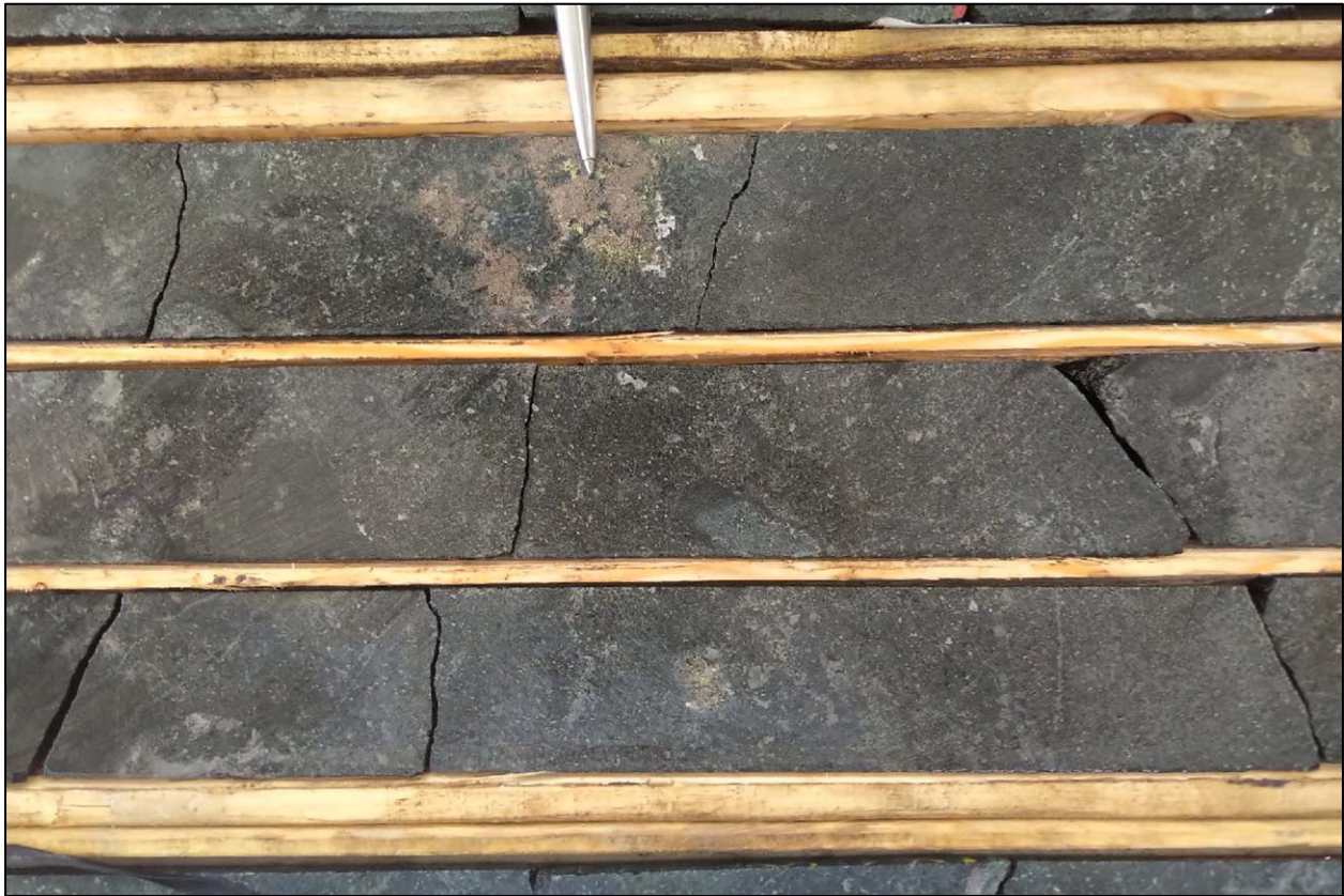
FIGURE 7.8 MINERALIZED INCLUSION RICH MELAGABBRO WITH LARGE GLOBULE OF CHALCOPYRITE-PYRRHOTITE IN DRILL HOLE EB21052, 239.5 M IN EOH ZONE
