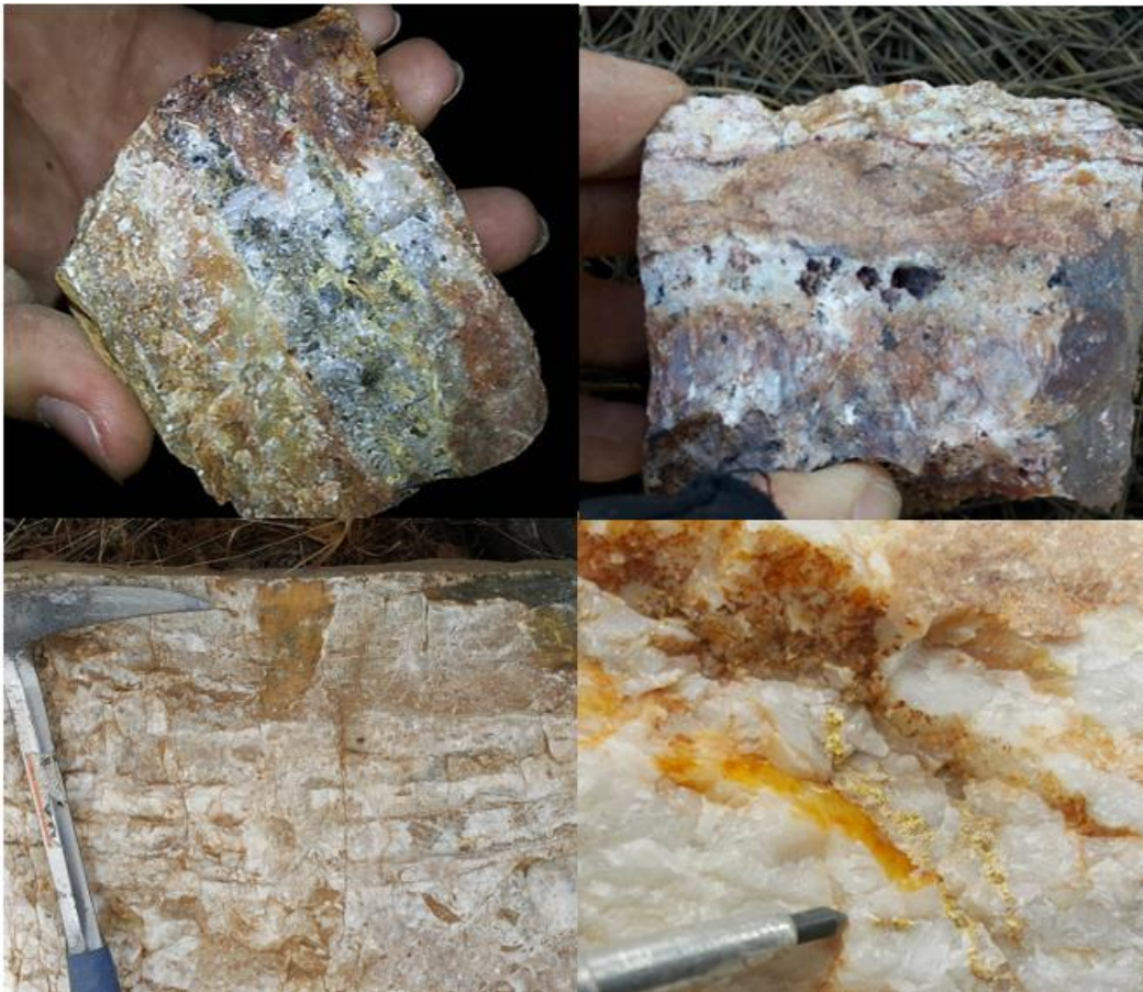
Figure 9: Photos of JOY East Property veins. Clockwise from upper left. 1. Quartz-sulphide vein with coarse sphalerite and minor galena. 2. Vuggy quartz vein with disseminated pyrite. 3. Weakly banded massive quartz. 4. Coarse visible electrum within massive quartz.
