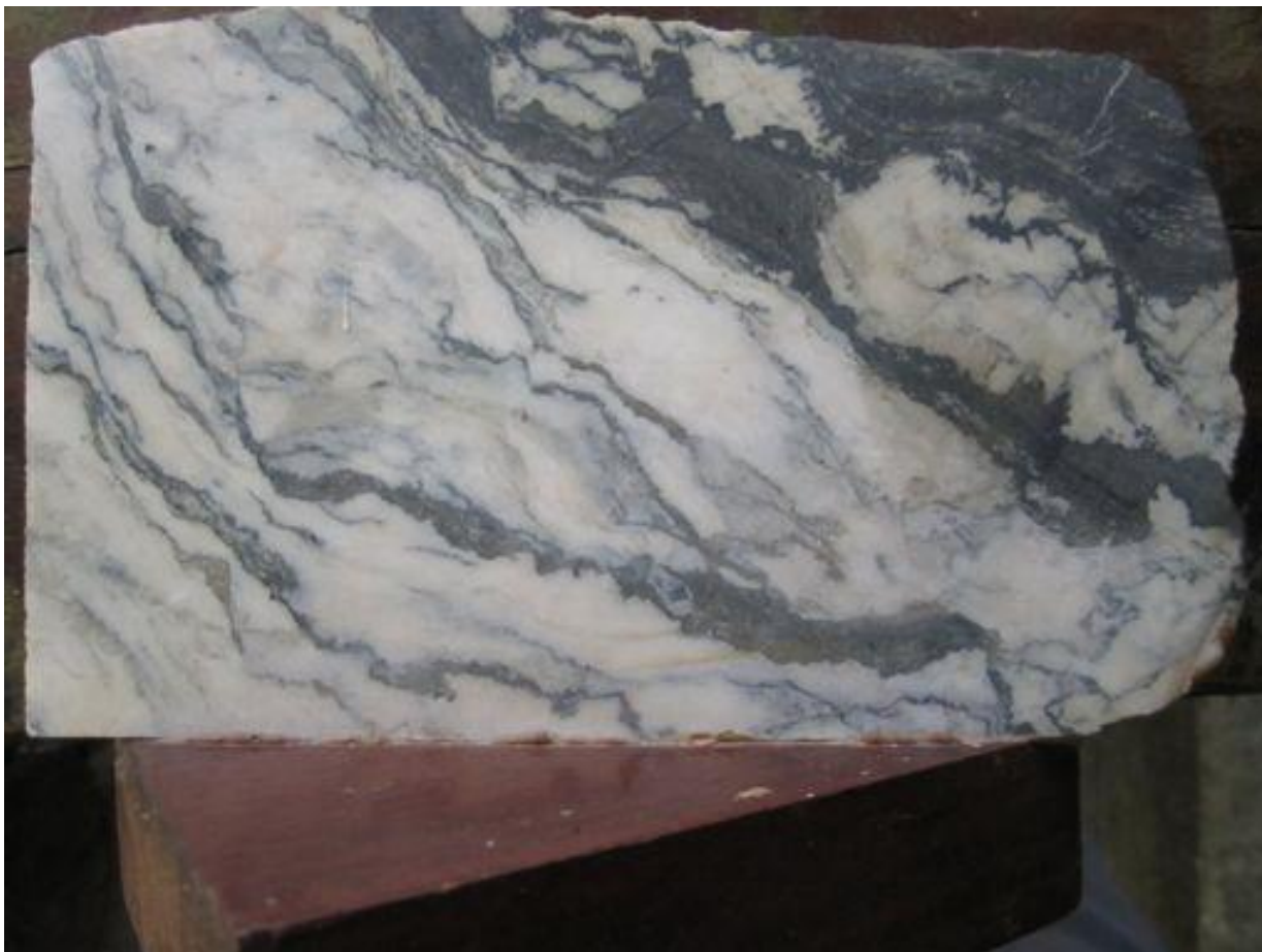
FIGURE 18. BOH YAI, TYPICAL MINERALISATION; PB-ZN-FE SULPHIDES IN SHEARED LIMESTONE
